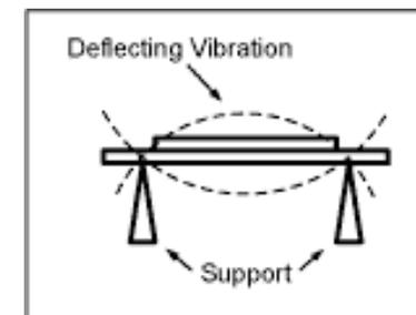
Oscillating voltage alternately squeezes and releases the piezo element. Must apply fluctuating voltage, a steady HIGH or LOW won't work.
