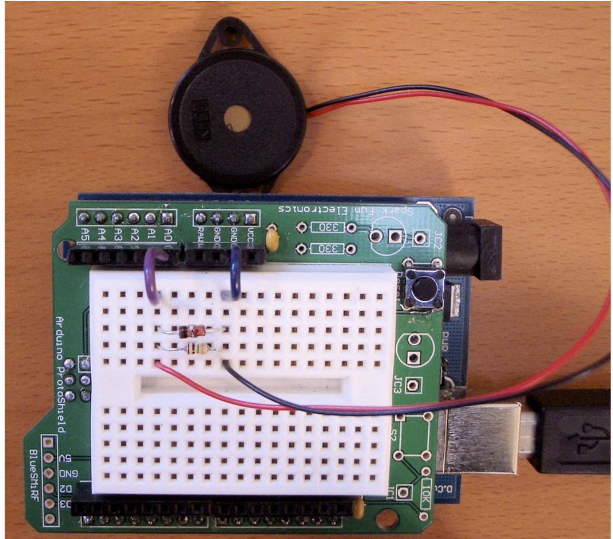
Create two little busses for GND and A0, and hook components across it. Black bar on diode indicates "bar" of diode.
