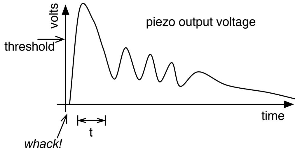
Depending on how fast you can watch the input, this technique works either really well or not that well. There are much faster ways of watching inputs that loops with `analogRead()`
