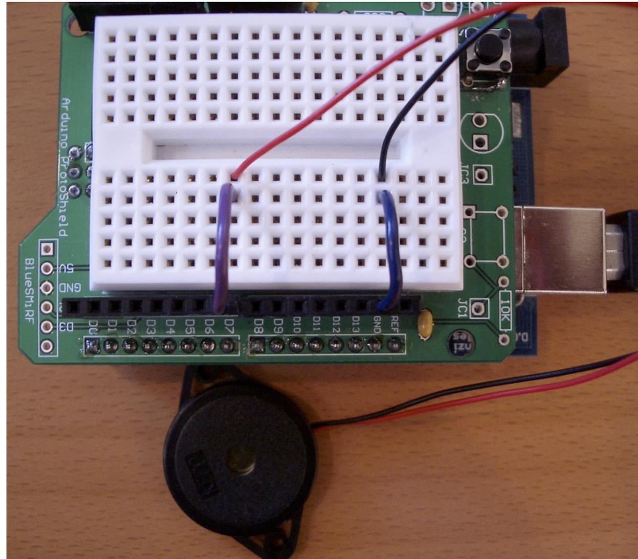
Piezo leads are very thin. The breadboard holes grab them better than the header sockets, which is why the jumper leads are used.
