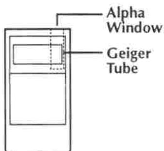
To measure as much as possible of the radioactivity of an object, place the Radalert 50 as close as you can without touching the object. The radiation level for gamma radiation from a localized source decreases according to the inverse square law. If you move to twice the distance from the object, the radiation drops by a factor of four.
