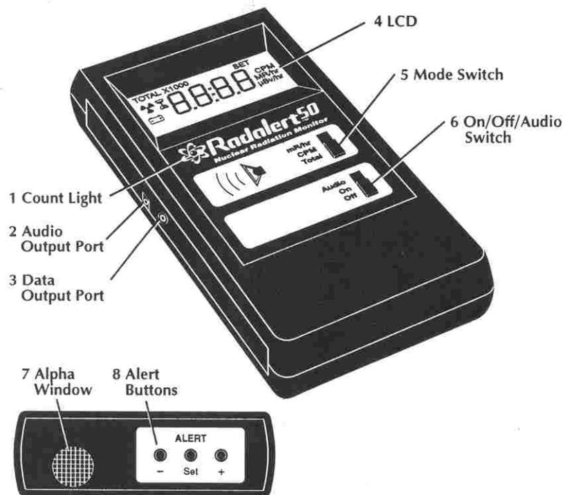
The Radalert 50 counts ionizing events and displays the results on the liquid crystal display (LCD) (4). You control which unit of measurement is shown by using the mode switch.
