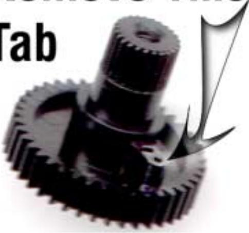
Removing the stop on the gear is only half the problem. There are still stops built into the potentiometer. You must now remove it as well.
